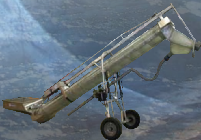
85 Class Ø 330mm 4,5m long loading elevator.
